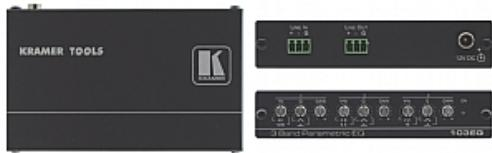
103EQ is a 3-band parametric equalizer that optimizes speaker sound quality, fixes microphone feedback and adjusts low, mid and high frequencies separately for precision sound customization. This compact-size equalizer was designed to make the Galil 2-C speaker fit the EN54-24 standard. For each frequency range, you can adjust the center frequency (Hz), bandwidth (Q factor) and gain (amplitude)
